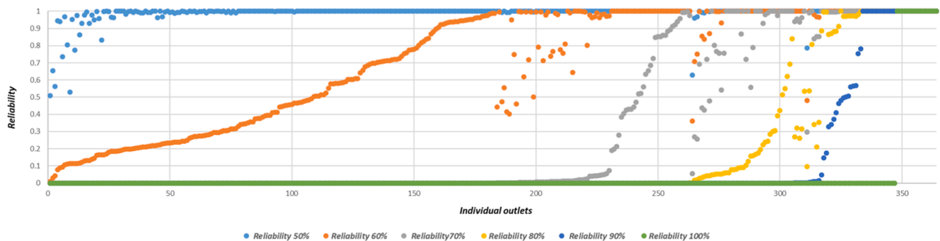
Fig. 5. Scenario S0. Reliability of individual outlets under different flow regimes, percentage of open outlets (50 – 100 %).
