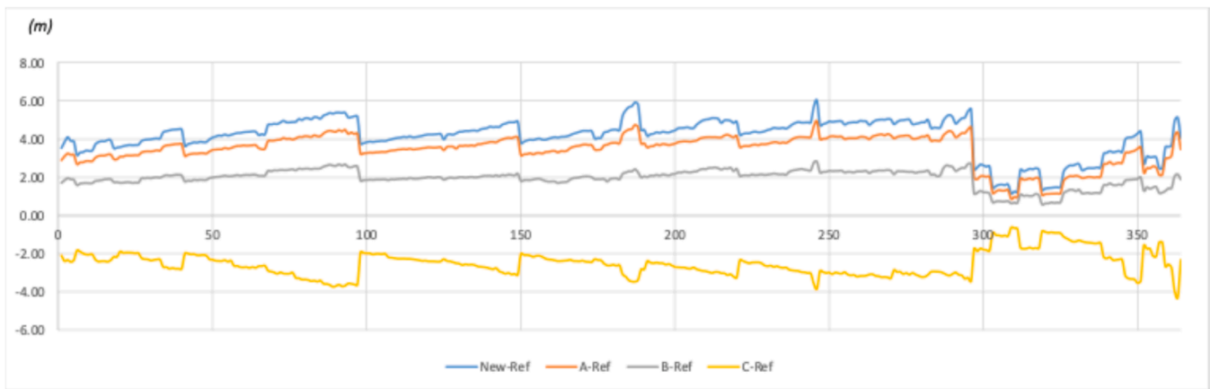
Fig. 14. Sensitivity of pressure computed at hydrants, in respect pipes roughness uncertainty. Values shown are average pressures computed at hydrants in cases New, A, B, and C minus computed average pressure in Ref case.
