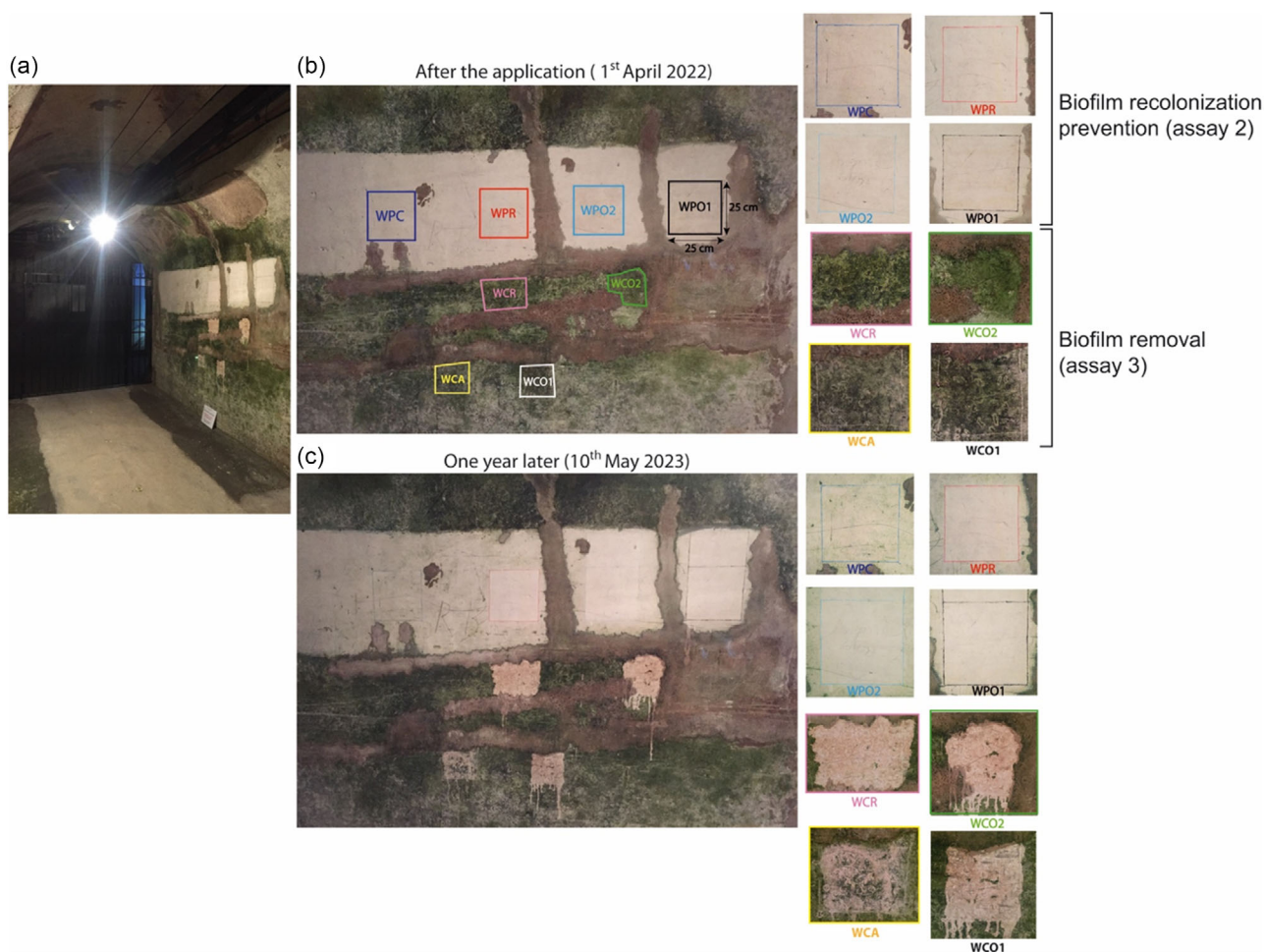
Figure 2. a) Photo of the illuminated corridor (12 h light/day) with biocolonized wall composed of chalk (white and green areas) and partially of cement (brown areas). A part of the chalky wall was cleaned for the biofilm recolonization prevention assay 2. b) Localization and zoom of control and treated areas on the cleaned wall for the biofilm recolonization prevention assay 2 and on the biofilm removal assay 3. c) Photo of the wall and zoom on areas of both assays 2 and 3 one year after application of products on the wall.
