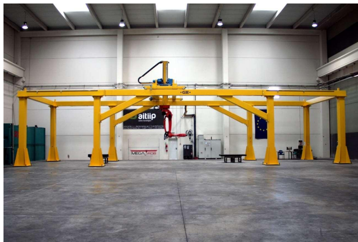
Figure 3. KRAKEN—Hybrid manufacturing robotic system. Photograph taken at the facilities of Fundación Aitiip.
