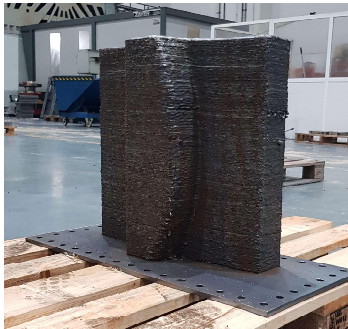
Figure 6. WAAM tooling printing over a metallic plate.
