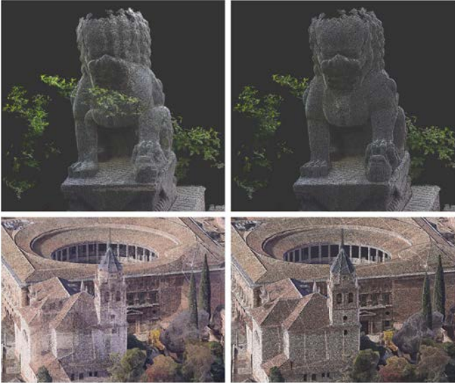
Figure 9. Point clouds rendered by a) deactivating and b) activating occlusion checks.
