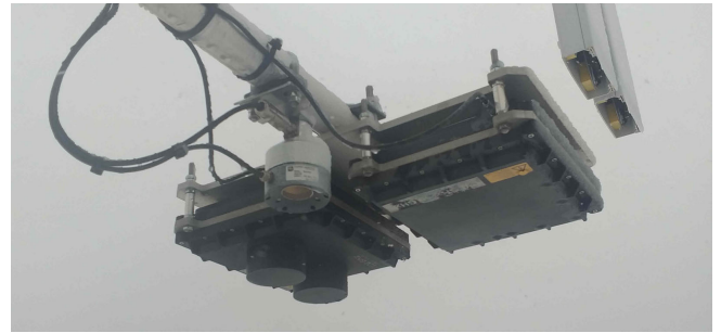
Fig. 3. (Bottom left) FMCW radar sensor installed at the AEMET-Formigal field laboratory. The sensor is housed within a protective plastic radome.
