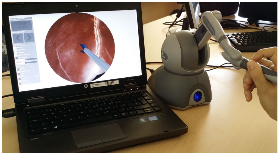
Fig. 5 The UniZar endoscopic surgery simulator, equipped with a Geomagic haptic device
