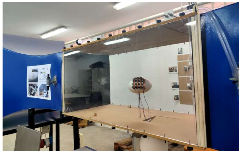
Figure 43. Sensor array validation using a wind machine.
