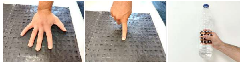
Figure 54. Representation of the validation technique with human subjects interacting externally with the device. Mat pressed by a hand ( left and center ) and mat integrated in bottle ( right ).
