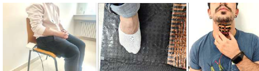
Figure 55. Representation of the validation technique with human subjects interacting externally with the device. Mat embedded in a chair ( left ), plantar pressure assessment ( center ) and mat externally attached to the neck ( right ).
