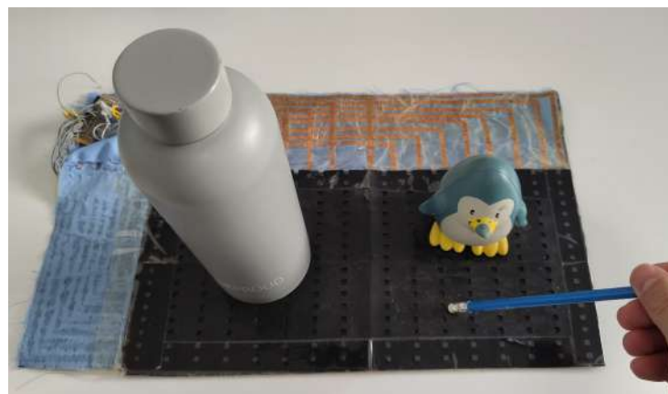
Figure 45. Sensor array validation using daily life objects.
