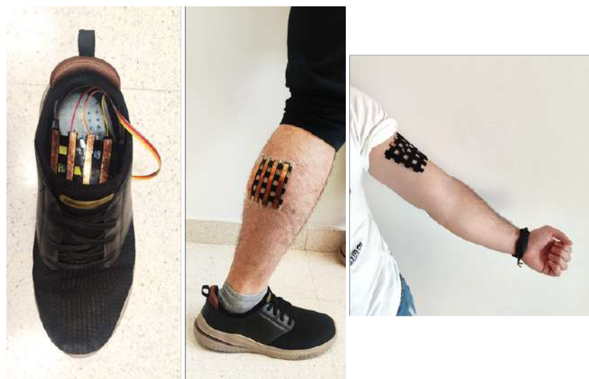
Figure 51. Representation of the validation technique with human subjects wearing the device. Shoe/foot (left), leg (center) and arm (right).
