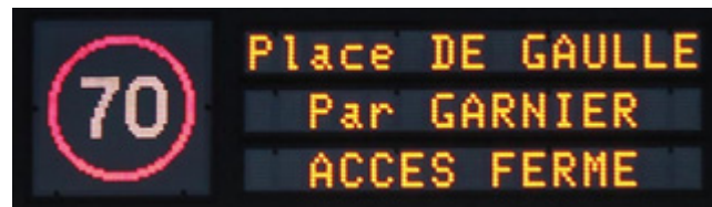
Figure 1. Example of a variable message sign (VMS) with two columns; one for pictogram and one for alphanumeric text (after Nouvier et al., 2009).
