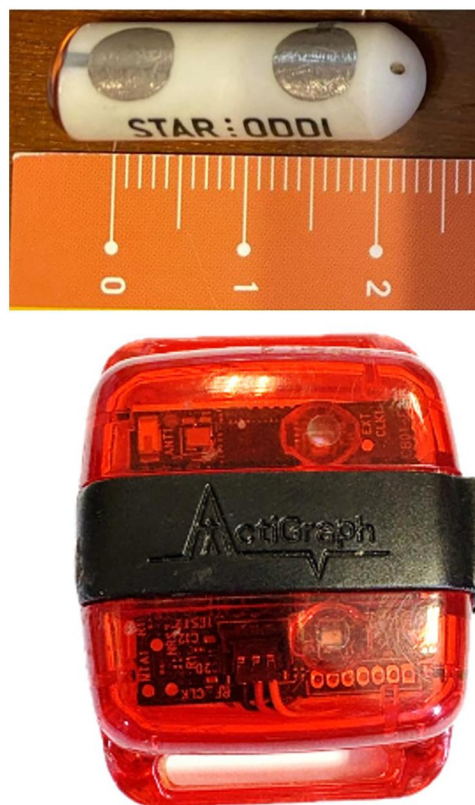
Figure 1. Subcutaneous biologgers ( 8.3 \times 25.4 mm; 3.3 g; DST micro-HRT, Star Oddi, Iceland) and triaxial accelerometers ( 46 \times 33 \times 15 mm, 19 g; ActiGraph wGT3X-BT, actigraph, Pensacola, FL, USA) that were used to record body temperature, heart rate, and heart rate variability, and locomotor activity, respectively, in lambs.
