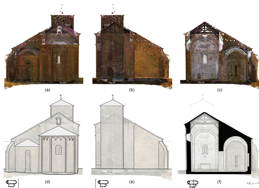
Fig. 10 Laser scan orthoimages: a) West elevation; b) East elevation; c) Transverse section. Elevation plans drawn from laser scan data: d) West elevation; e) East elevation; f) Transverse section (Source: the authors)
