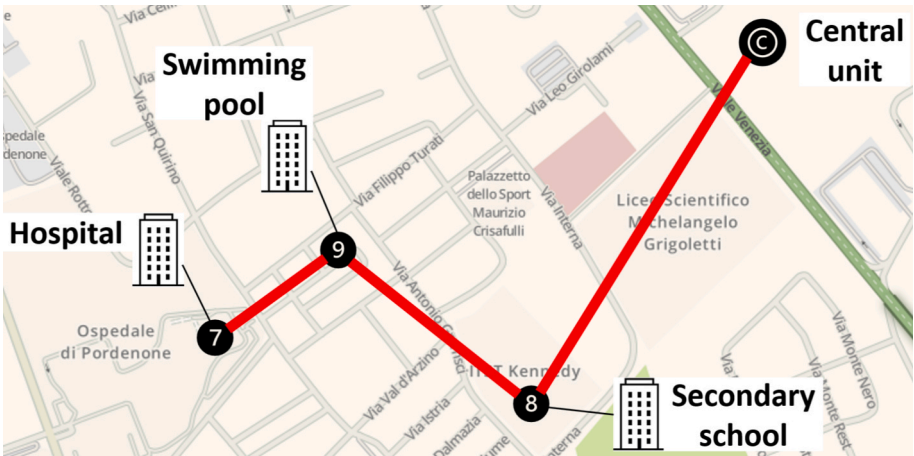
Fig. 16. Optimal economic solution: DHN pipeline connections between buildings 7, 9, 8, and central unit.
