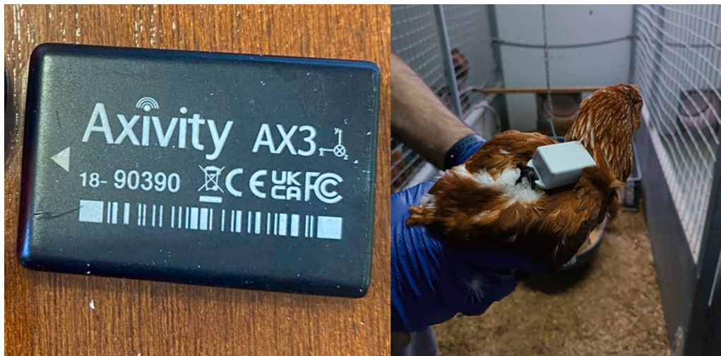
Fig. 1. Laying hens ( n = 5 ) were fitted with commercially available tri-axial accelerometers (Axivity AX3 3-Axis, 23 \times 32.5 \times 7.6 mm; 11 g) that recorded raw acceleration data, which were housed in a plastic box (Hammond ABS, 50 \times 35 \times 20 mm, 18 g) that was attached to a dorsal harness.
