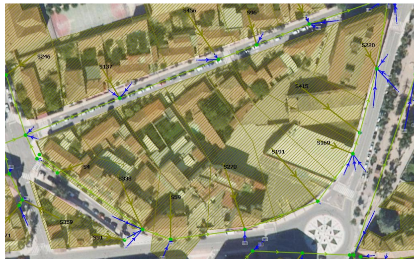
Figure 2. Extract of subcatchments in the residential area (light brown hatched polygons) and the connections to the nearest manhole (green nodes). Light brown arrows represent the connexion of subcatchments to manholes and blue arrows represent the connexions of inlets to manholes.
