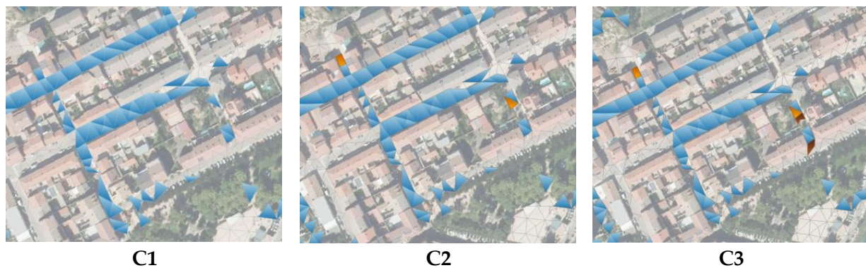
Figure 10. Increase in flood extend with inlet clogging patterns C1, C2, and C3. Mesh elements in blue represent flood depth above 1 cm for clogging scenario C1; orange and brown represent the increasing of flood extent (mesh elements) for clogging scenarios C2 and C3, respectively.
