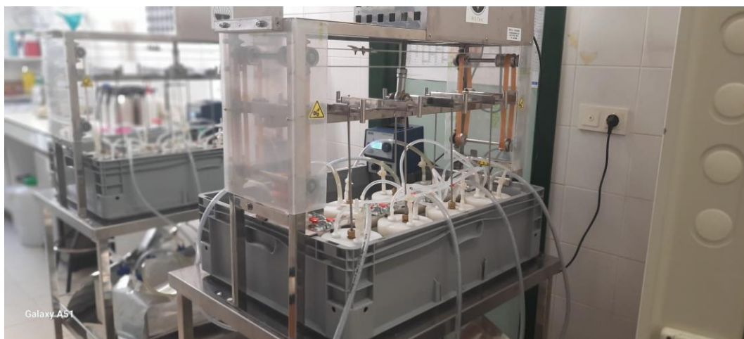
Figure 11: Rusitec system at the laboratory of Animal production at the faculty of Veterinay (University of Zaragoza).
