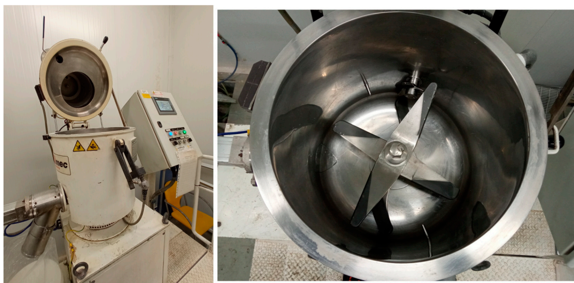
Figure 2. Turbo-mixer for the adsorption process of active compounds onto silica.
