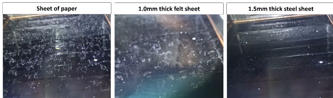
Figure 9. Tests with different barriers between the cathode ray tube and the cloud chamber.
