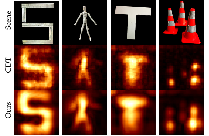
Fig. 6. Reconstructions of real world measures scenarios. Each column represents a different scene. Top: photographs of the scenes behind the diffuser. Middle: Lindell and Wetzstein reconstructions [17] (CDT). Bottom: our reconstructions using phasor fields. The higher-frequency of CDT is related to the deconvolution to compensate scattering at the diffuser.
