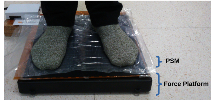
Fig. 4. Picture showing the configuration of the PSM and the FP in the human stability tests.
