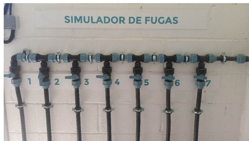
Figure 4. Valves for leak simulation. The numbering of the valves is directly related to the representation of the leak points in Figure 2.
