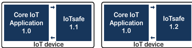
Fig. 5. Upgrading IoTsafe on an IoT device: IoTsafe stand-alone security modules interface with the core IoT Application through local sockets, easing security upgrading processes thanks to software independence [15].
