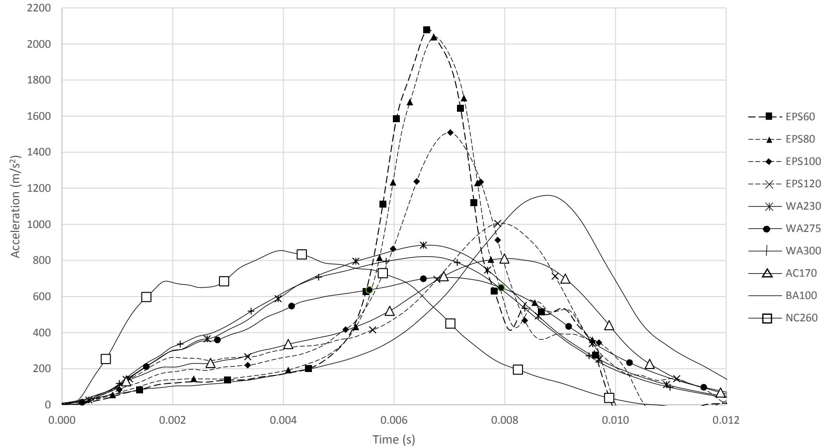
Fig. 8 Deceleration (m/s<sup>2</sup>) - time curve for corks and cork products for the 75 J dynamic test. Specimen:
