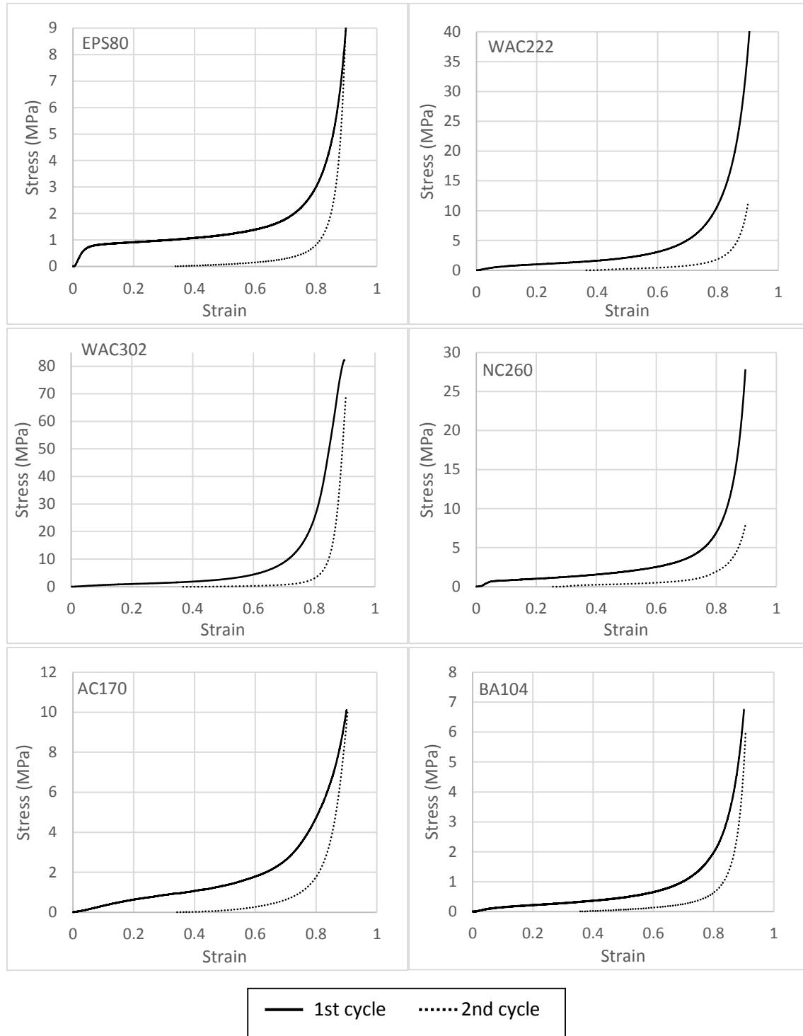
Fig. 10 Stress-strain curve for some of the studied materials under two consecutive load cases with a maximum strain of a
