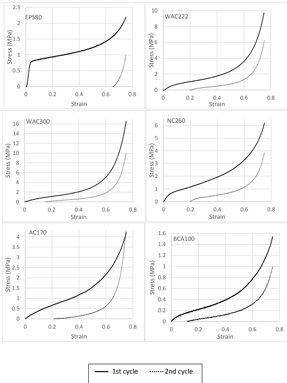
Fig. 11 Stress-strain curve for some of the studied materials under two consecutive load cases with a maximum strain of a
