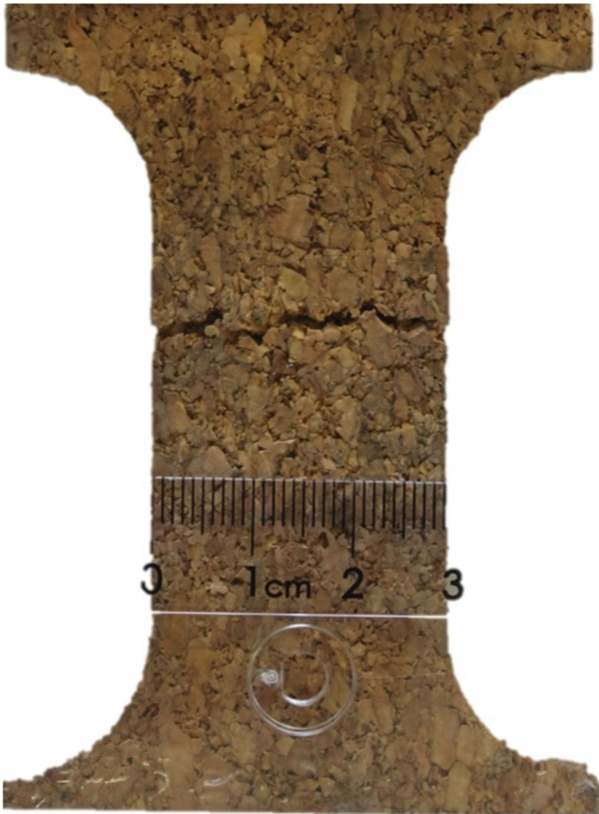
Figure 7. Brittle failure of the WC275.
