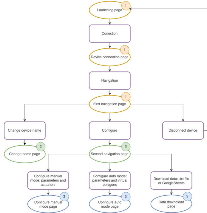
Fig. 1. Reduced logic app design. Functions: purple; Screen 1: yellow. Screen 2: green; Screen 3: blue.
