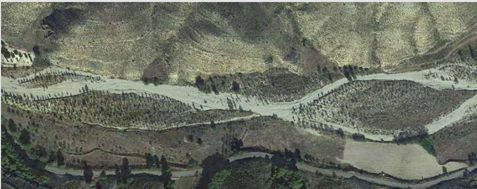
Figure 90. Islands stabilised by plantations in the Barranco de la Nava (Aguilar del Río Alhama, La Rioja).
