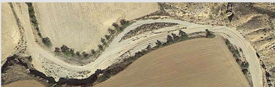
Figure 81. The frequent passing of vehicles has caused two channel-bend shortenings in the Rambla de la Alhóndiga (Terrer, Zaragoza).
