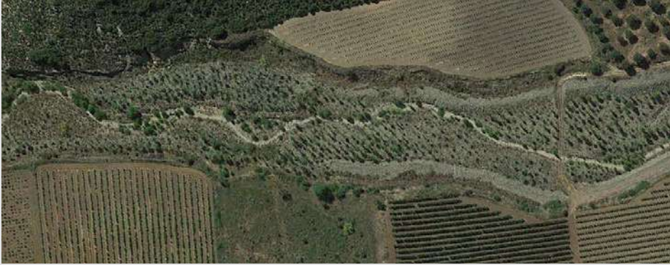
Figure 89. Upper-middle reach of la Yasa Agustina stream (Autol, La Rioja) with plantations in the channel, increasing active bed incision.
