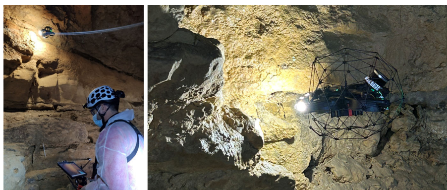
Figure 6. Data acquisition and inspection workflow using the confined-space UAV, integrating LiDAR–SLAM navigation with simultaneous video capture for videogrammetry.
