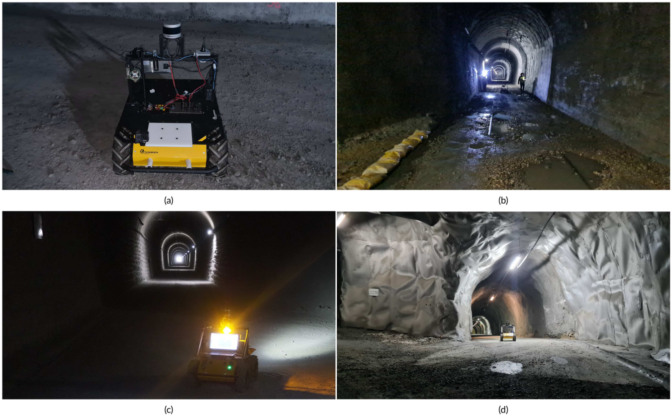
FIGURE 22 | Pictures taken inside the Somport tunnel during our experimental run. a) Close-up of our robotic platform, a Clearpath A200 equipped with a VLP-16 LiDAR sensor. b) Picture taken from the intersection of G7 with the main tunnel, where the floor is especially rough. c) Picture taken in the main tunnel, between G8 and G7, it can be seen that the tunnel walls present few geometric features. d) Entrance to G8 seen from the main tunnel. [Color figure can be viewed at wileyonlinelibrary.com ]
