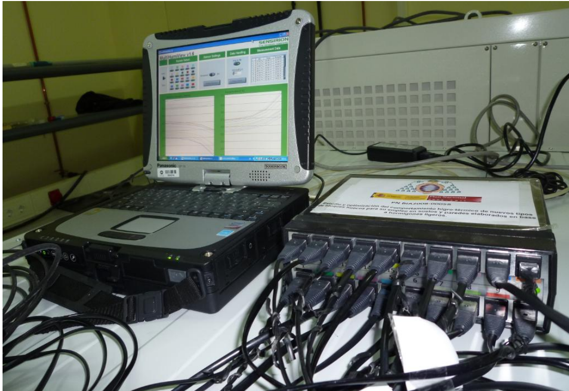
Fig. 6. Data acquisition system from temperature and humidity sensors type SHT75.
