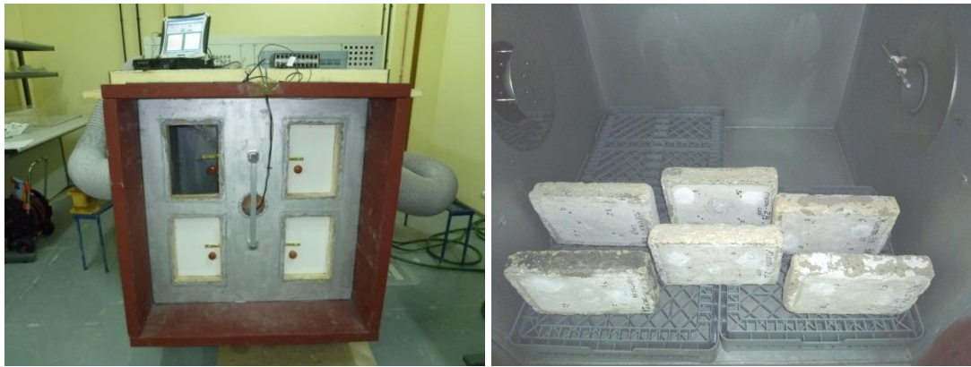
Fig. 4. Experimental setup (left) and specimens located inside the hot-box test chamber (right) for hygroscopic tests.
