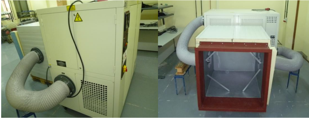
Fig. 3. Photographs of the climatic chamber (left) and hot-box apparatus (right).
