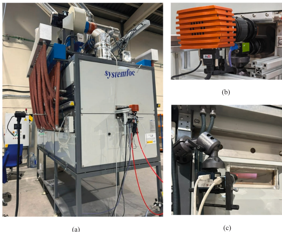
Fig. 2. (a) Furnace chamber, (b) camera setup from the front view with the Raptor Photonics Falcon Blue and the Jai GO-5000-PGE, (c) camera setup from the side view with the Imaging Source DFK 33GX174 and the EHD-704UV.
