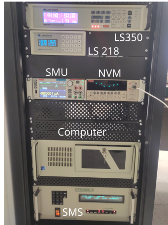
Figure 3.3.: The CFMS rack equipped with the measurement electronics.
