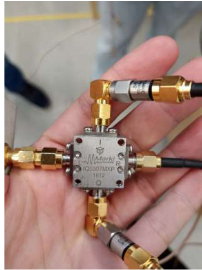
Figure 6.16: IQ mixer used for some of the measurements presented in this work.
