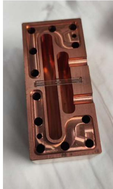
Figure 7.4: Left : Aluminium double cavity. Right : Copper double cavity with transmon installed, transparent sapphire substrate can be seen in the centre.
