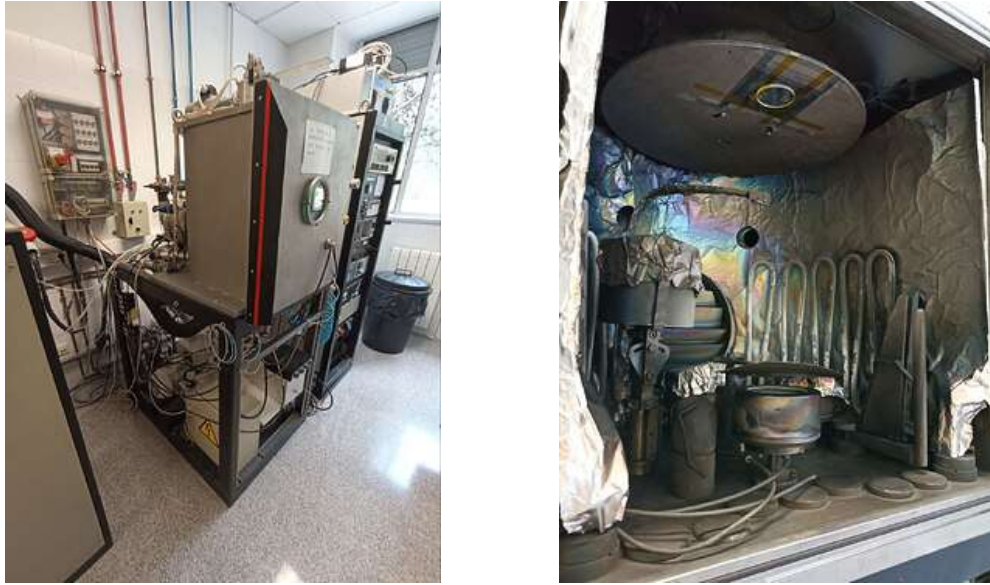
Figure 4.3: Left : General view of the thin layer deposition equipment. Right : interior of the sputtering oven. The sample can be seen hanging from the ceiling.
