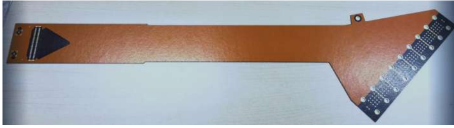
Figure 3.8: Flat cable for Micromegas V2 made of copper and kapton.
