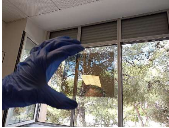
Figure 4.5: Glass sample used as a test for the deposition of the thin aluminium layer. Here transmission and reflection images for visible photons can be seen in the sample.
