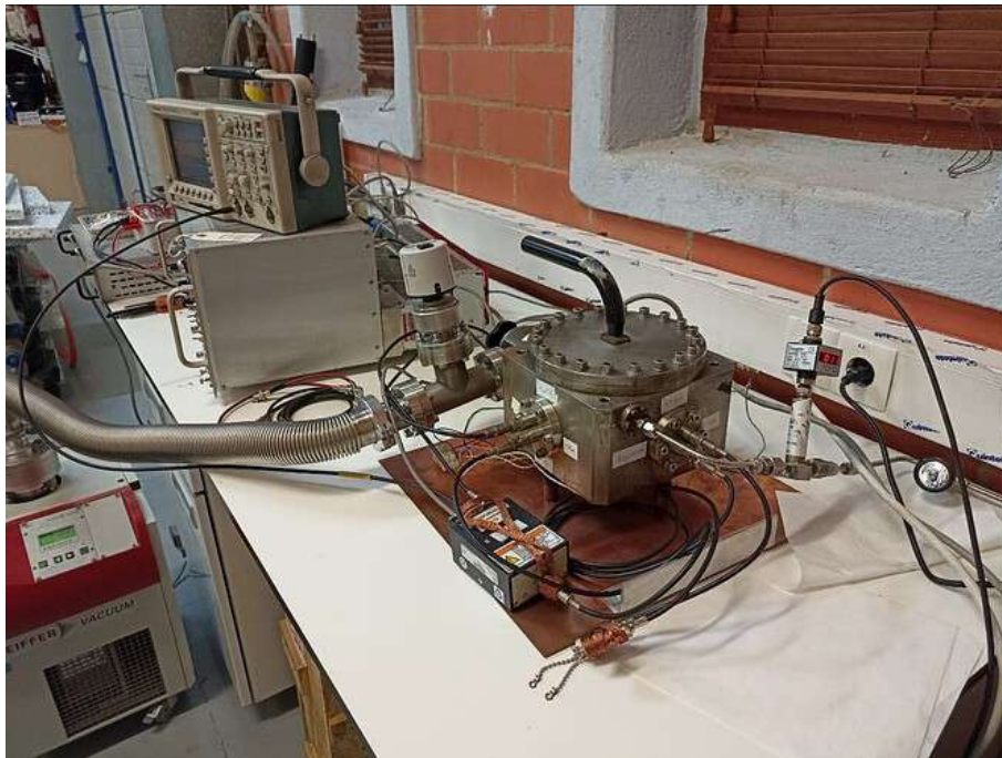
Figure 4.12: General view of the setup for argon + 10% isobutane measurements. The chamber with preamplifier and pressure sensors in foreground, oscilloscope and power supplies in the back.
