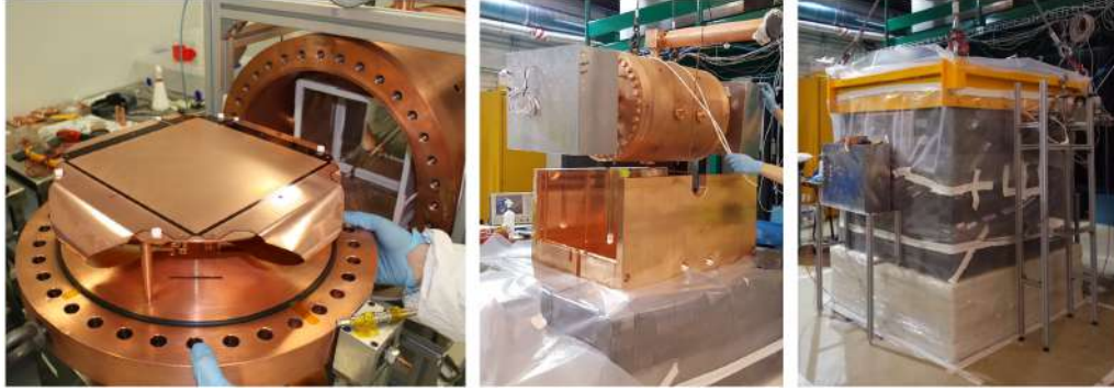
Figure 3.2: Left: Micromegas readout plane attached to one of the end caps. Middle: Closed vessel about to be placed inside the shielding. Right: TREX-DM is installed and operating in Hall A of the LSC. The lead shielding surrounding the chamber and the lower part of the polyethylene neutron shielding are visible [64].
