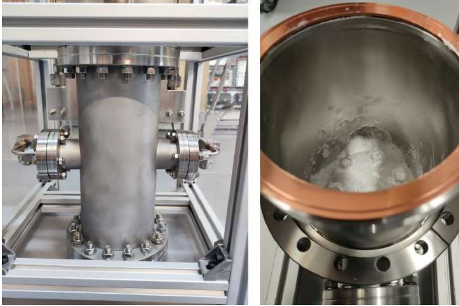
Figure 3.45: Left : Vessel for CaO powder. Right : 0.5 kg of CaO powder inside the vessel.
