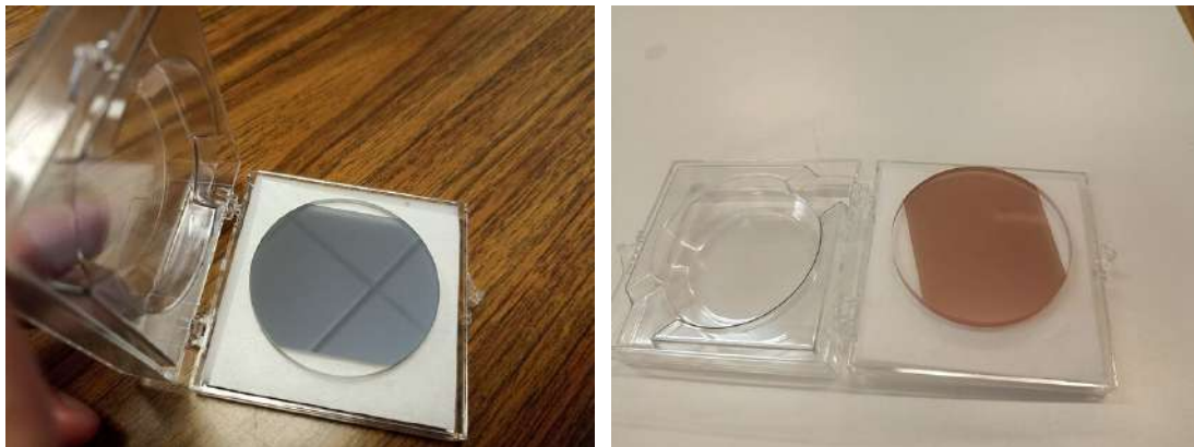
Figure 4.4: Photocathodes, made of thin metallic layers over a quartz substrate. Left : 30 nm thickness aluminium layer. Right : 20 nm thickness copper layer.
