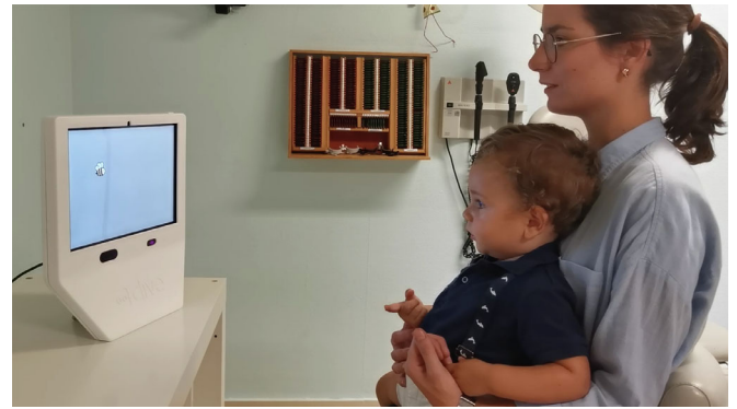
Figure 1. DIVE being used by a young patient sitting on his mother's lap. DIVE includes a Huawei Matebook E tablet with a 12-in. tactile screen and an integrated X3-120 Tobii eye tracker.
