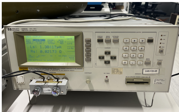
Figure 5.1. Agilent 4284A LCR meter.
