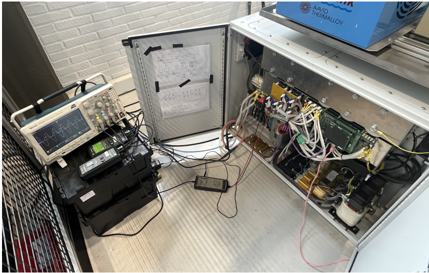
Figure 5.17. Voltage and current waveforms measurement setup with Tektronix MD03054 oscilloscope.
