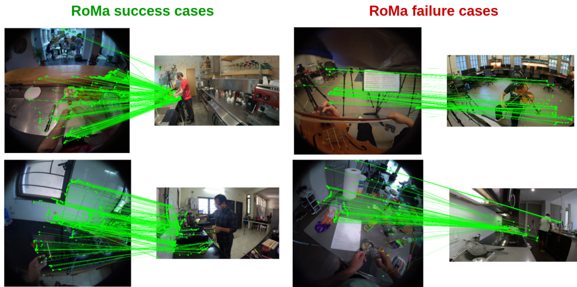
Figure 8.5: RoMa success and failure cases. The extreme view variance makes that, even SOTA methods in geometry matching like RoMa [2], fail in extracting matches.
