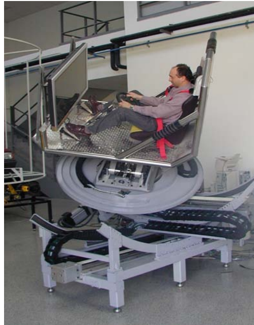
Fig. 14. Central control station's motion base
