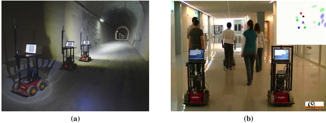
Figure 3.1: Example of applications of robot formations developed at University of Zaragoza. (a) Formation deployment inside a road tunnel. (b) A triangle-shaped robot formation guides a group of people towards the exit during a building evacuation.
