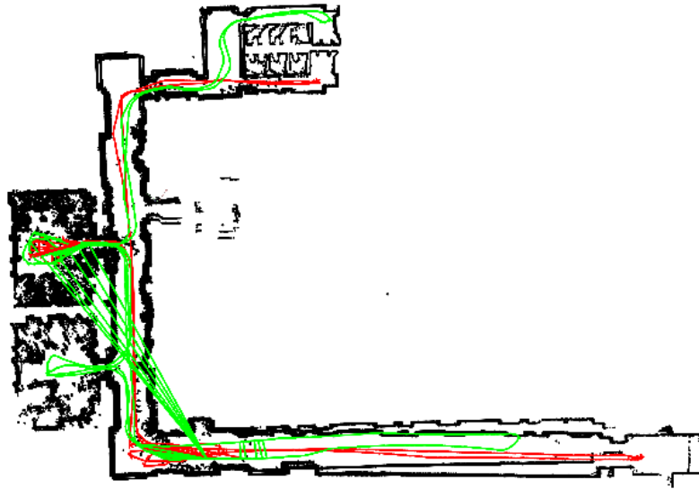
Figure 7.13: Experiment at the DIS building of La Sapienza University of Rome. The misalignment observed in the bottom right corner originates from the fact that the robots never meet in that region, thus they are unable to determine constraints between that part of their trajectories. This can be recovered when the two robots meet in that region, or in a post-processing phase.
