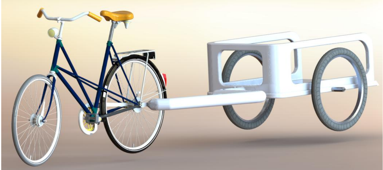
Figure. 1.17. Trailer attached to the rear wheel.
