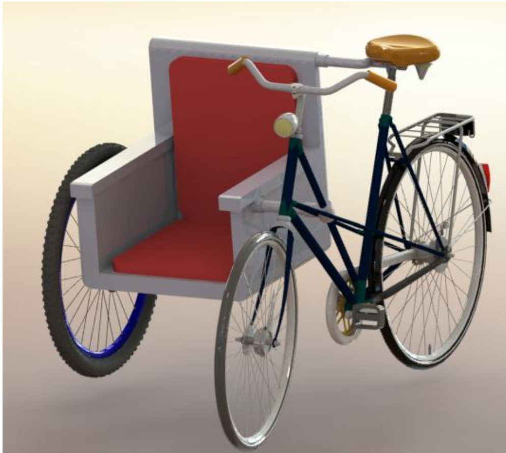
Figure 4.2. Especial trailer designed for being a sidecar.
