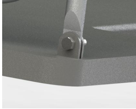
Figure 1.26. The bar and the trailer are joint through screw and nut assembly.
