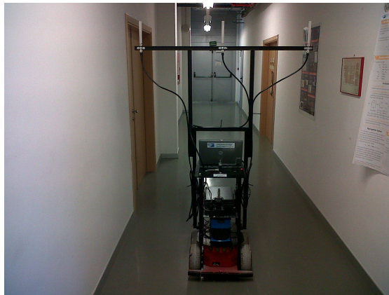
Figure A.2: Coverage mapping tool based on Pioneer 3-AT robot.
