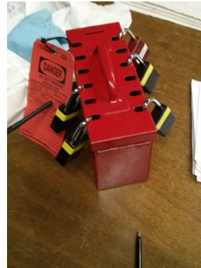
(b) Locked box with the penstock activation key
