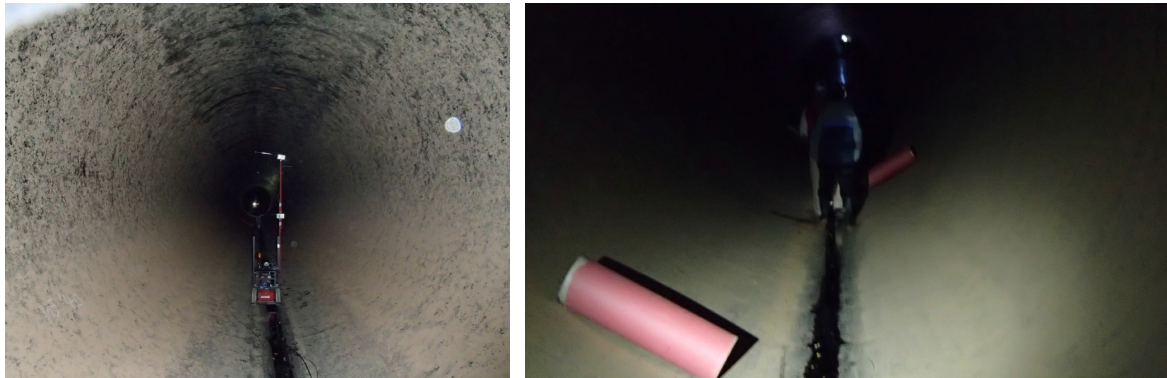
(a) Instrumented Pioneer P3AT robot inside the large-scale pipe
