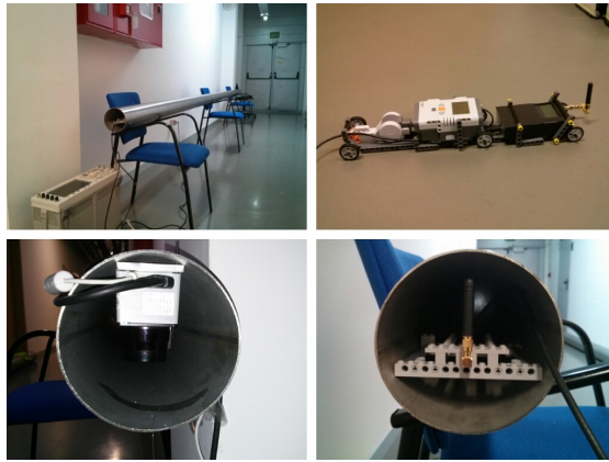
Figure 2.3: Laboratory experimental setup. From upper left, clockwise: the small-scale pipe, the receiver robot, the transmitter platform, and the the laser sensor for position estimation.
