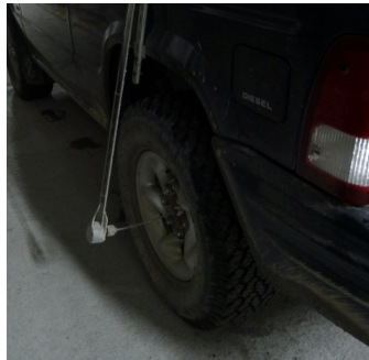
Figure A.5: 0.5 degree resolution wheel encoder from ATv2.
