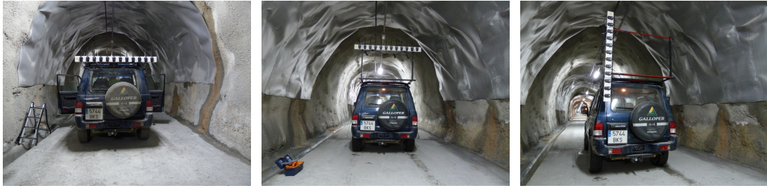
(a) Horizontal receivers at a height of 2 m. (b) Horizontal receivers at a height of 3 m. (c) Vertical receivers
