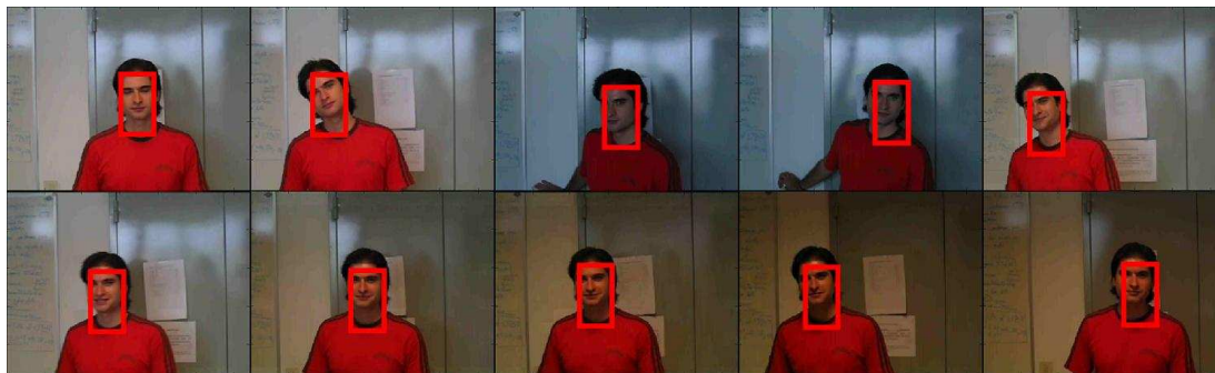
Figure 4.25: Tracking face with illumination changes using RBPF and non-parametric model. Frames:2, 36, 85, 119, 185, 196, 214, 217, 223, 279, 319.
