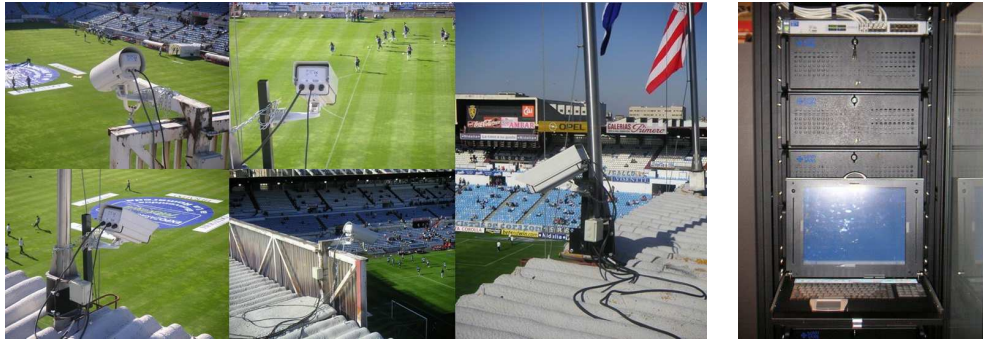
Figure 5.11: Installed cameras and processing cluster.
