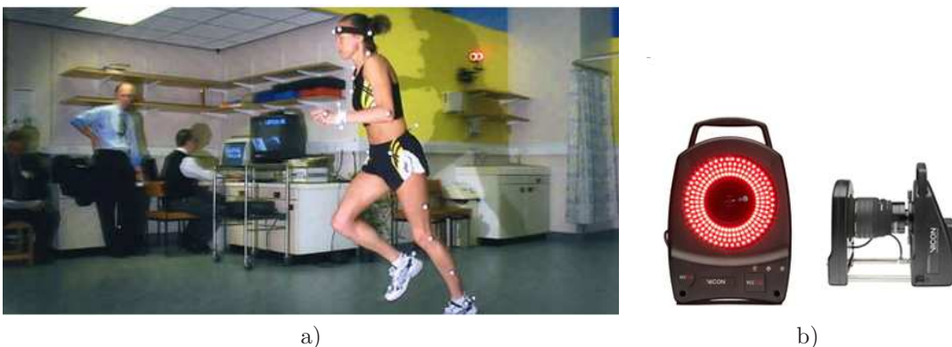
Figure 2.5: VICON Motion capture system. a) Example of application. b) Detail of infrared cameras used in the system. (Image source: http://www.vicon.com )
