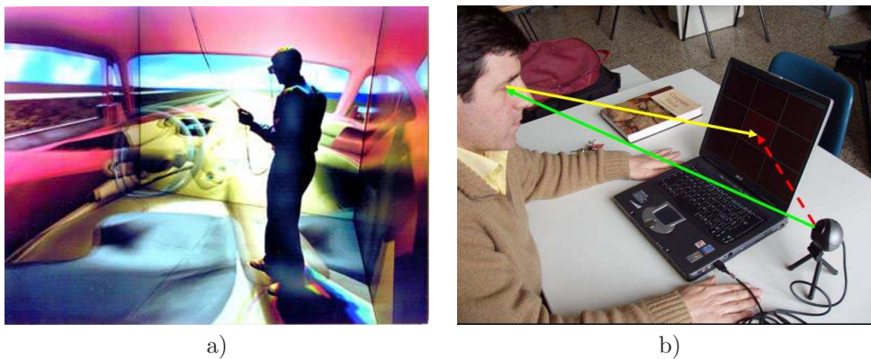
Figure 2.7: Examples of human-machine interfaces: a) CAVE virtual reality system. b) Eye-mouse using webcam. (Image source: http://um3d.dc.umich.edu/hardware/CAVE/ and http://vcg.isti.cnr.it/~corsini/research.html )
