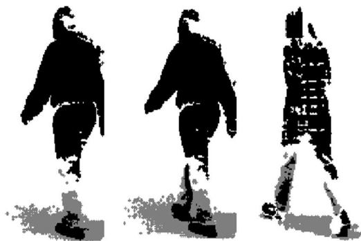
Figure 3.10: Results of applying the shadow removal. Shadows in gray
