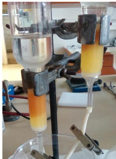
Fig 14. Dowex resin cleaned by NaOH.
