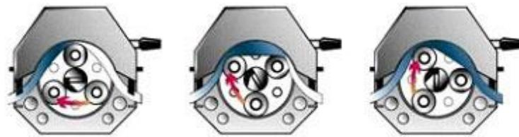
Fig 8. Peristaltic pump process [31].
