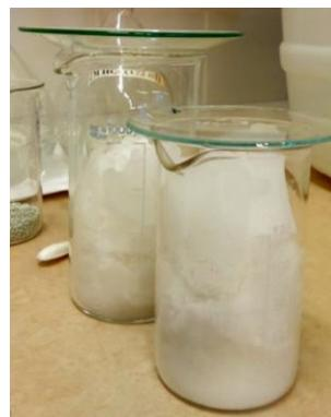
Fig 16. Sephadex resin cleaned by water in three steps.
