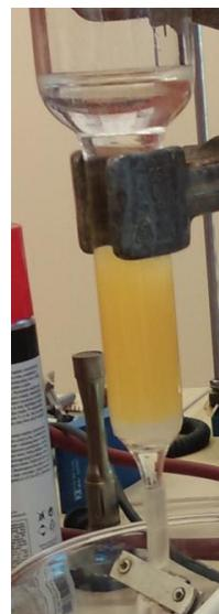
Fig 13. Dowex resin cleaned by HCl.
