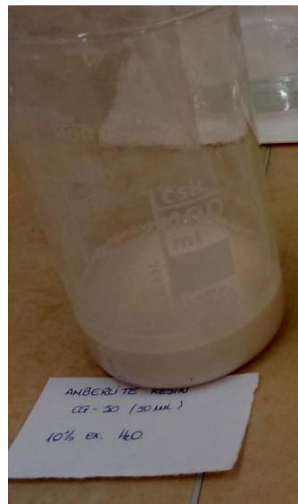
Fig 11. AMBERLITE CG50 resin cleaned by water.
