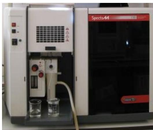
Fig 10. Varian SpectrAA 200 atomic absorption spectrometer. [35]
