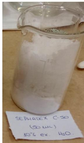
Fig 15. SEPHADEX C-50 resin cleaned by water.
