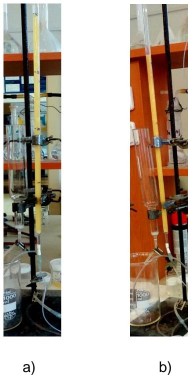
Fig 18. Resin column used in experiments. Picture a) shows 40 mL of resin in the column and picture b) is the same column with less length of resin beads.
