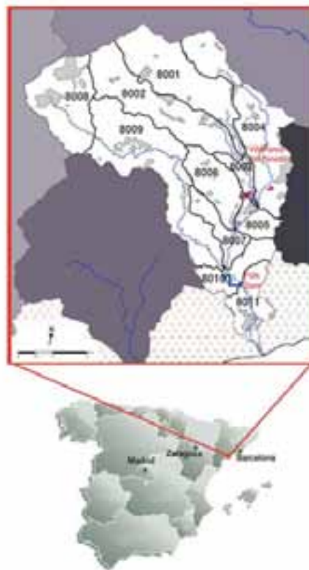
Figure 7.3. The Foix watershed, showing eleven sub-basins used in the spatial and temporal emergy evaluation of resource values of water. Grey shadow indicates the main urban areas, while pink colour represents the industrial ones.
