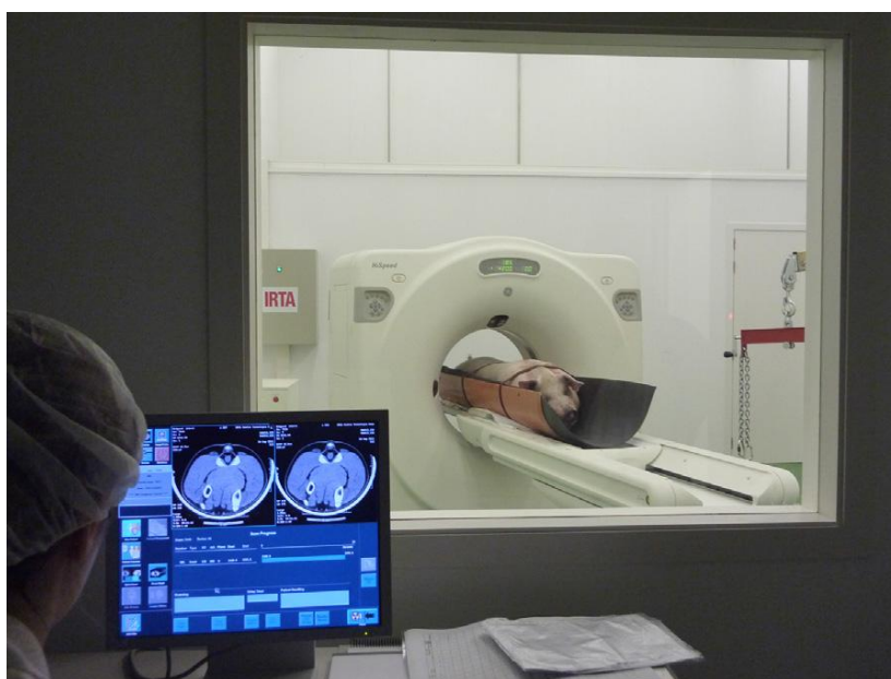
Figure 1. Evaluation of live pigs with the computed tomography machine.
