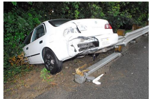
Figure 3. Accident due to the beginning of the steel barrier. [4]
