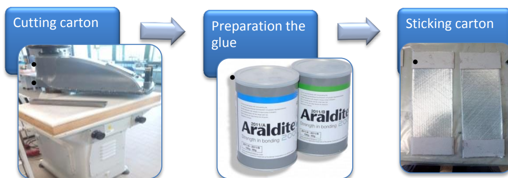
Figure 3.13: Steps for preparing trial before uniaxial test
