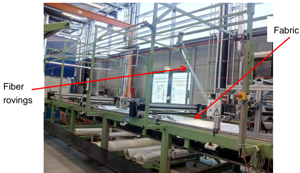
Figure 2.9: Copcentra MAX 3 CNC with additional fiber chopper device [ITA]
