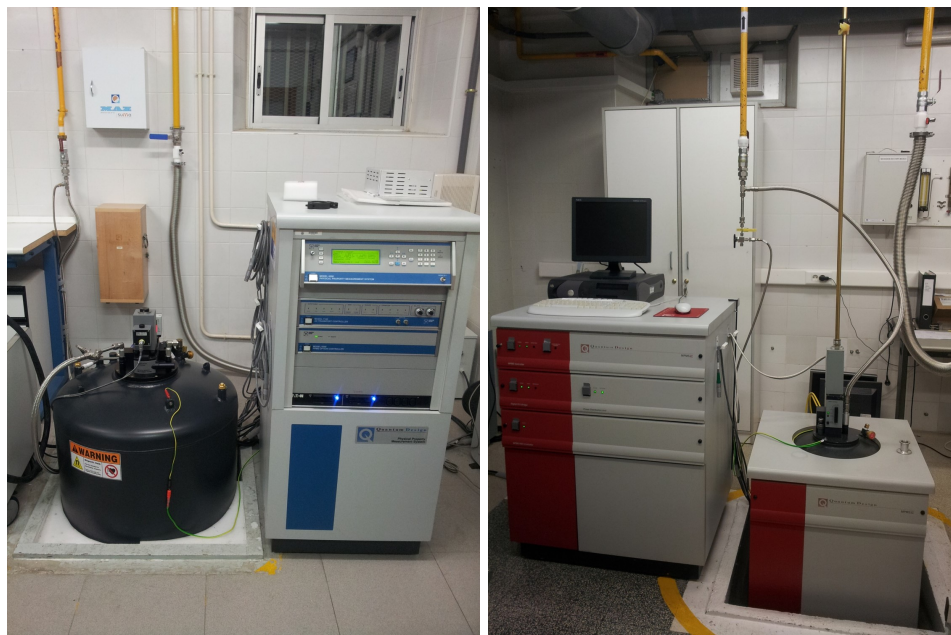
Figure 2.1: PPMS (left) and MPMS (right) equipments.
