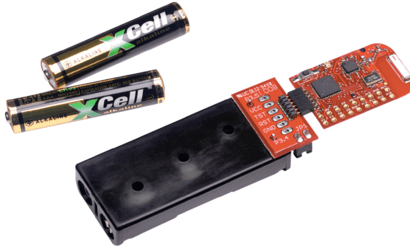
Figure 2. eZ430-RF2500 Battery Board
