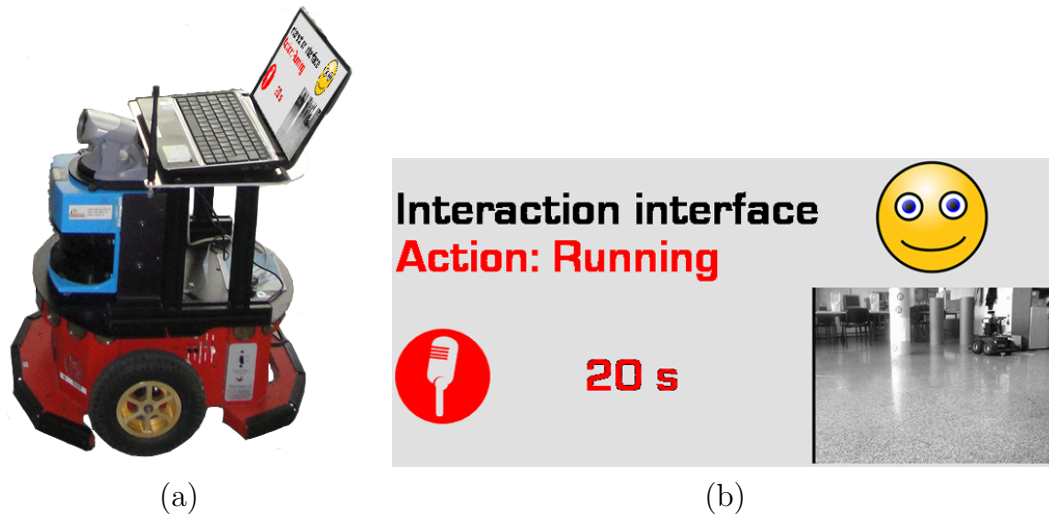
Figure 4.3: (a) Robot device in the brain-actuated redesigned telepresence system with a laptop placed on it. (b) Graphical interface of the robotic system.
