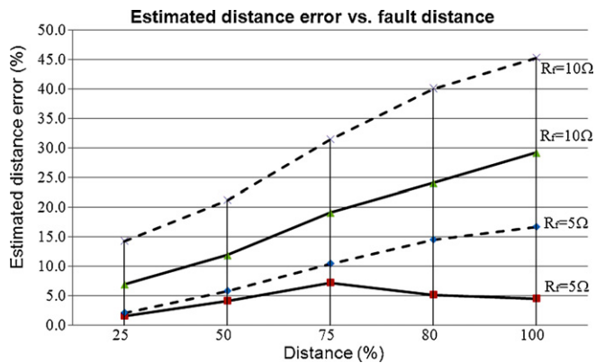
Fig. 12. Comparison of the distance errors by DEA using filtering application (solid lines) and without (dashed lines) for 5 and 10 \Omega fault resistance simulation.
