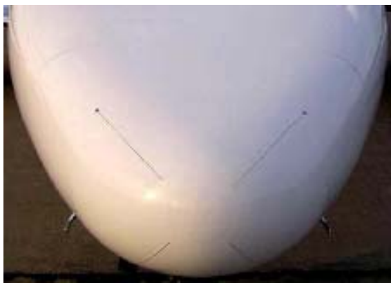
Figure 5.2.1.1.1 Diverter stripes on the nose [9]
