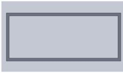
$$\begin{aligned} h &= 4000 \text{ mm} & I &= 4.71 \cdot 10^{12} \text{ mm}^4 \\ b &= 5000 \text{ mm} & W &= 2.35 \cdot 10^9 \text{ mm}^3 \\ e &= 100 \text{ mm} & A_c &= 8 \cdot 10^5 \text{ mm}^2 \end{aligned}$$
