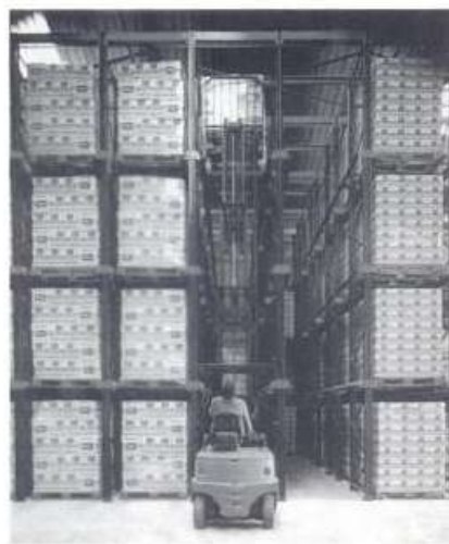
Figure 3.a – compact shelving palletization. Source: ([Maul03] p.16)
