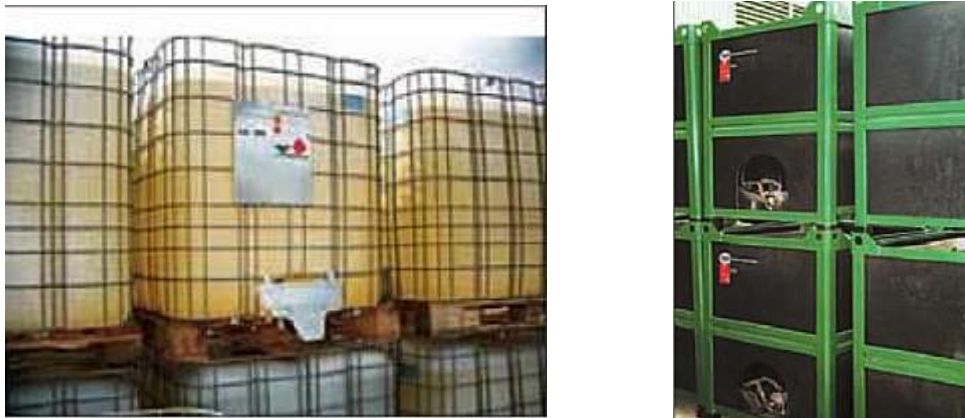
Figure 13- Different types of IBC (intermediate bulk containers). Source: ([Gome09], p.61)
